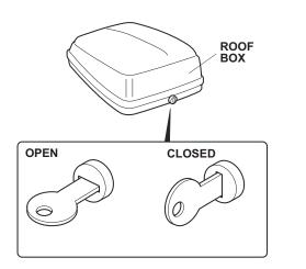
**Locking:** Press down on the lid. You should hear a click. Be sure the lid is latched by attempting to lift the lid. Turn the key clockwise to lock the roof box. Remove the key while not in use. Be sure the straps are not outside the roof box.
